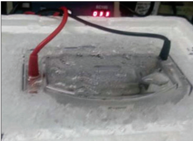
Figure 1: A submersed electrophorator. Figure 7 from 'Western Blot: Technique, Theory, and Trouble Shooting'. [1]
