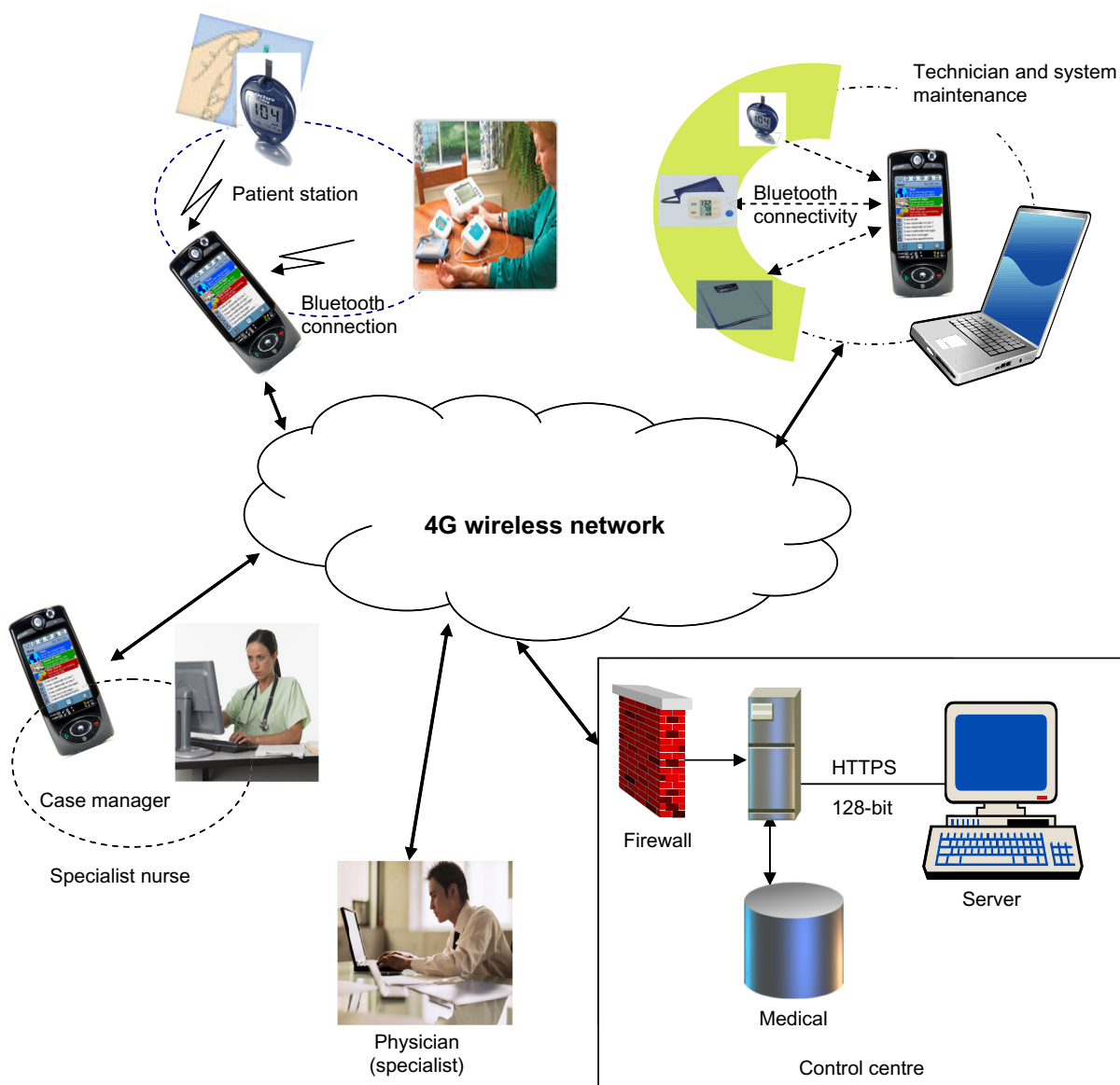
Figure 1 Schematic representation of a home (fixed) and smartphone (mobile) telemonitoring systems showing the key relationships between the patient technical and medical/nursing health professionals.
