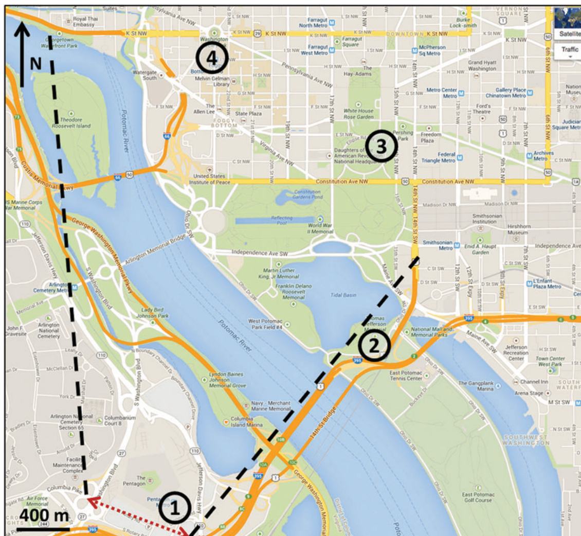
Figure 2. Predicted downwind dispersion areas and sample collection locations for 2009 release. The approximate release location is shown by the red dotted line. The black dashed lines show the boundaries of the predicted downwind dispersion area. The high-volume air sampler locations are shown as circles; environmental samples were collected in the immediate vicinity of the air samplers.
