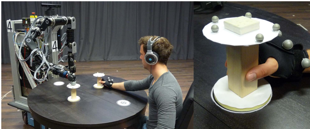
Figure 11. Experimental setup. Left: The scenario of a prototypical joint pick-and-place task. Right: Hand movements are made available to the robot in real time by tracking the glove the human interaction partner is wearing. doi:10.1371/journal.pone.0095195.g011
