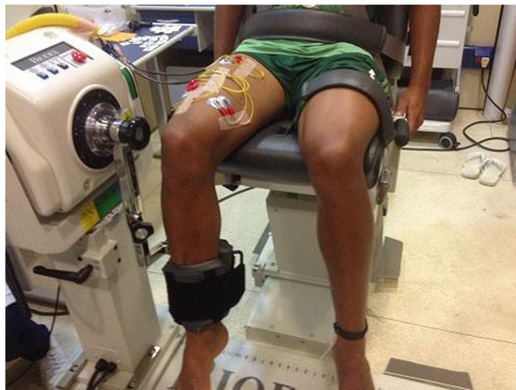
Figure 7 Experimental setup employed to record the EMG and the torque.
