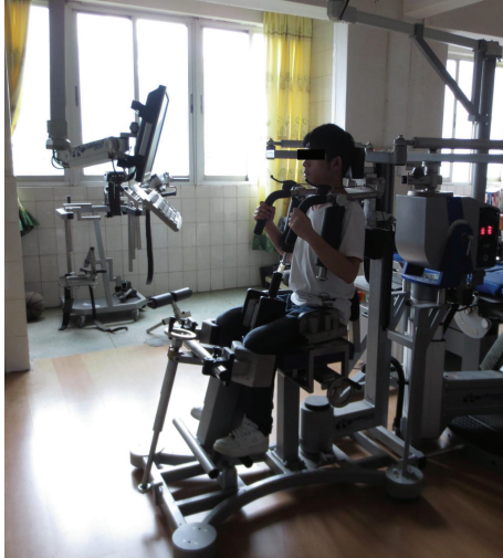
FIGURE 1: Subject was seated in the Isomed 2000 Torso Rotation isokinetic dynamometer for trunk rotation testing.
