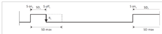
Figure 8. Example of how stimulus duration is determined by response (R) (Pre-Ballot Draft ISO 17488).
