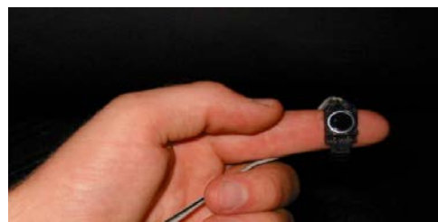
Figure 6. Finger-mounted buttons used to record reaction time (adapted from an early draft for NWI ISO 17488)
