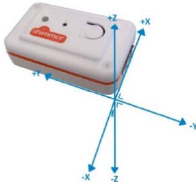
Figure 3. Coordinate system of the kinematics sensor [32].
