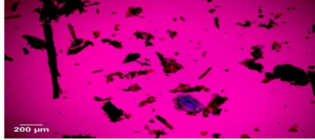
b Acid pretreated bagasse or Cellulignin (20 \mu\text{m} )
