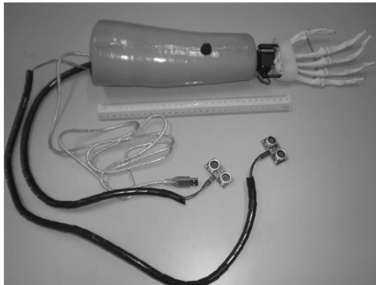
Figure 1 New development of the biomechanics wrist prosthesi using ultrasonic sensors as the input, servo motors as the output and microcontroller.
