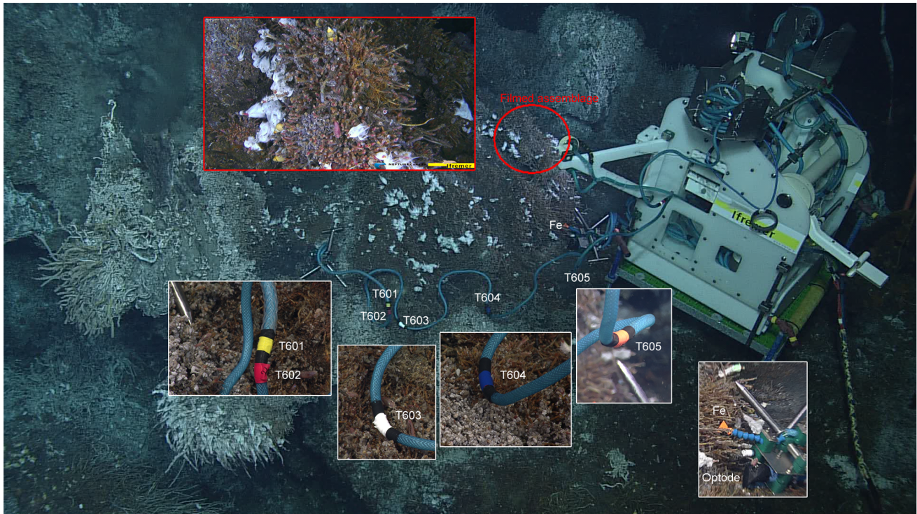
Figure 2. TEMPO-mini module in situ . TEMPO-mini in situ , at Grotto hydrothermal vent at 2186 m depth. Insets show the filmed assemblage as well as the deployed environmental probes. T60x were the temperature probes and CHEMINI Fe and optode sampling inlets were mounted on a tripod deployed below the filmed assemblage. doi:10.1371/journal.pone.0096924.g002
