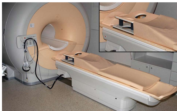
Figure 1 Magnetic resonance imaging scanner with closed bore magnet and a dedicated 8 channel phased-array breast coil (top right). Technically any magnetic resonance imaging scanner could be used in breast image acquisition. However, in daily practice, field strengths of 1.5 T and 3 T are often used due to higher spatial resolution at similar temporal resolution, providing better diagnostic efficacy.
