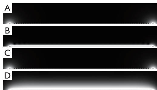
Figure 4 Simulated images for planar SEA array, with different phase offset between neighboring channels. By manipulating the phase shift across nearest neighbors, the transmit field slice thickness can be varied. The phase offset was set to be (A) 0^\circ , (B) 180^\circ , (C) 20^\circ and (D) 340^\circ . SEA, single echo acquisition.
