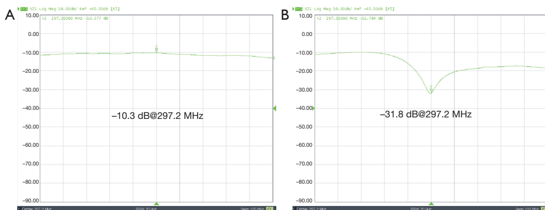
Figure 5 Measured S_{21} plots vs. frequency of two monopole elements loaded with the water phantom. (A) Without the decoupling element; (B) With the decoupling element. The isolation between the two elements can be reduced from about -10 dB to about -32 dB, indicating the strong decoupling ability of the ICE/magnetic wall method for the monopole array.
