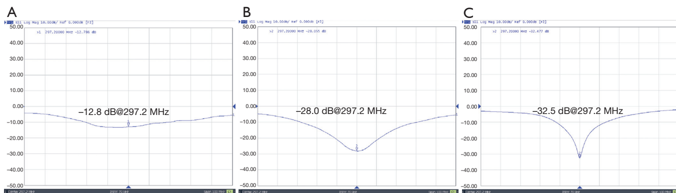
Figure 4 Measured S_{11} plots of two monopoles loaded with the water phantom. (A) Without matching circuits and without the decoupling element; (B) With matching circuits and without the decoupling element; (C) With matching circuits and the decoupling element. The S_{11} of the coil elements could be improved to better than -28 dB with matching circuits added, indicating the monopole elements were well matched by using the L-shaped capacitive networks.
