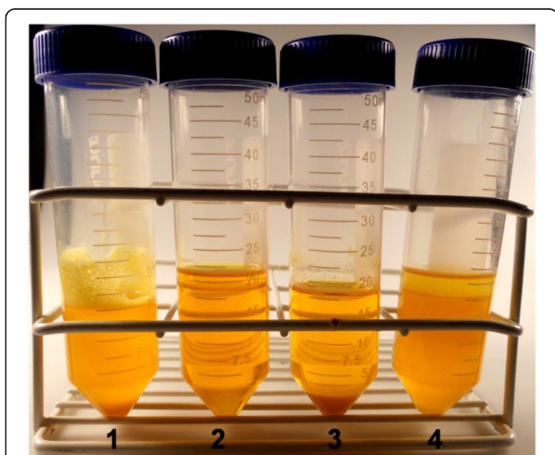
Figure 2 Dissolving effect of methanol on oil gums. (1) Soybean oil (raw material); (2) soybean oil with 1.5 eqs MeOH; (3) soybean oil acid degummed; and (4) soybean oil acid degummed with 1.5 eqs MeOH. Image obtained after 24 h incubation at 35°C, 250 rpm agitation, and centrifugation at 2,000 rpm for 5 min.
