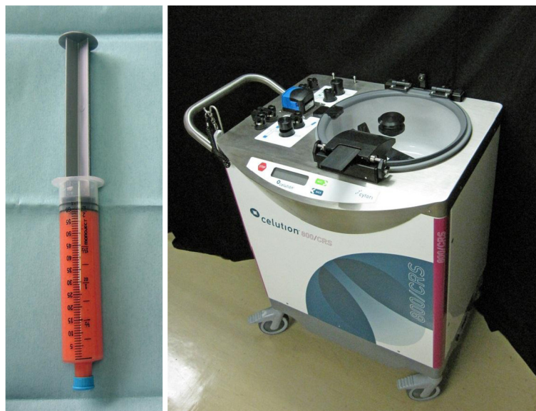
Figure 1 Human abdominal subcutaneous fat (left) was applied to the Celution®800/CRS (right) to extract ADRCs.
