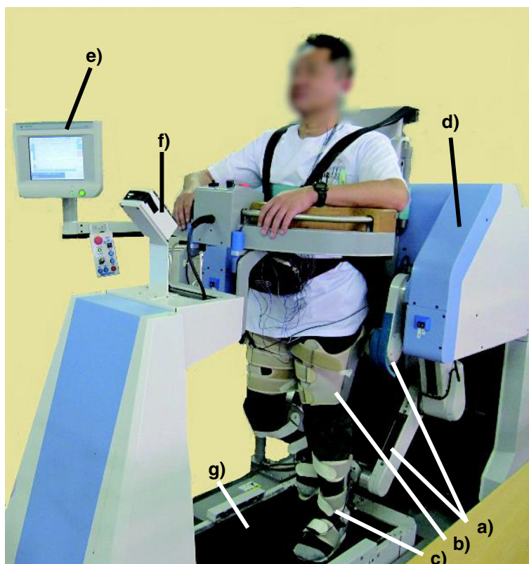
Figure 1 Gait-Assistance Robot. The Gait-Assistance Robot consists of a) 4 robotic arms for the thighs and lower legs, b) thigh cuffs, c) lower leg apparatuses, d) a generator, e) a control panel, f) lights for the foot pressure biofeedback system, and g) a treadmill.
