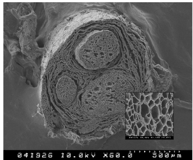
Fig. 2 Electron microscopy image of AxoGen processed acellular nerve allograft demonstrating internal microstructure (courtesy of AxoGen, Inc.)
