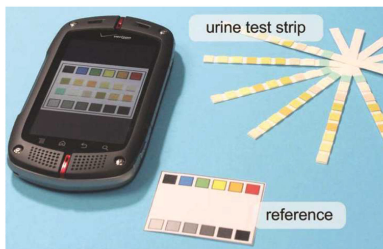
Fig. 8. Cellphone-based technique for colorimetric measurements in urine test strips [31]. Reproduced with permission from the Royal Society of Chemistry.
