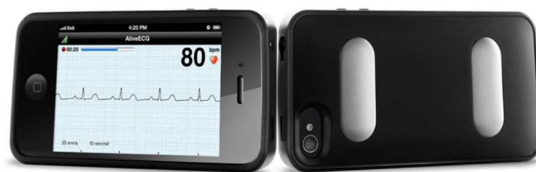
Fig. 9. AliveCor's Heart Monitor [32]. It is an FDA approved device that has recently been cleared for sale in US for use by medical professionals to record, display, store, and evaluate single-channel electrocardiogram (ECG) rhythms. Reproduced with permission from David McCaman, AliveCor, Inc.
