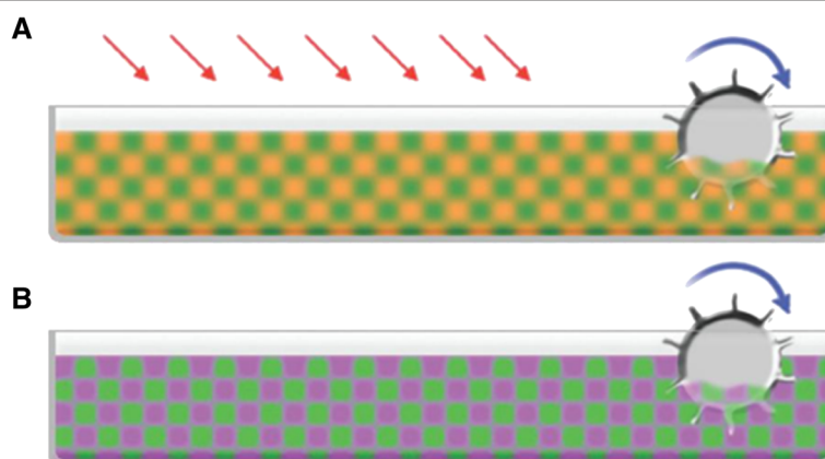
Figure 4 Control of biological contamination. A. Chemicals (red arrows) are released into the culture medium in order to combat biological contamination (orange) in an open system containing microalgae (green). The circle represents the blades turning at low speed for system circulation. B. Controlled management of allelopathy-derived compounds (magenta) from microalgae (green) eliminating biological contamination in open-pond cultivation. The circle represents the blades rotating at low speed for system circulation.
