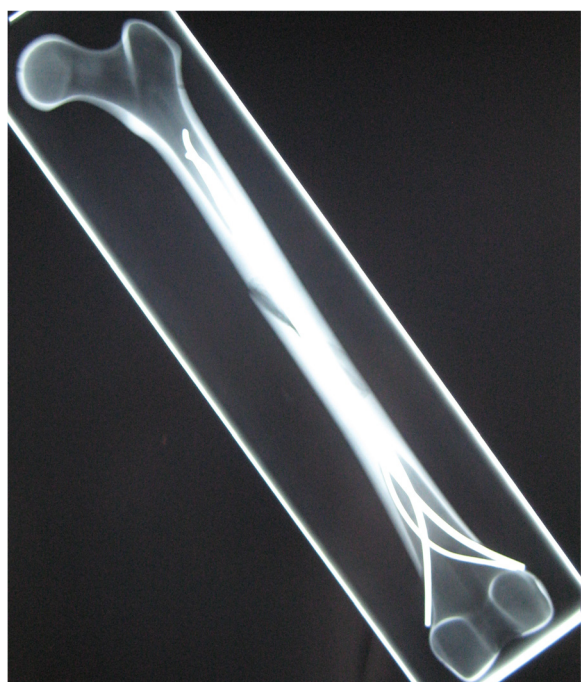
Figure 1 Radiograph (anterior-posterior view) of a 3CL femoral model with retrograde intramedullary nailing, showing two 3.5 mm titanium nails implanted in 2C shaped configuration and one additional 2.5 mm titanium nail implanted antero-lateral.
