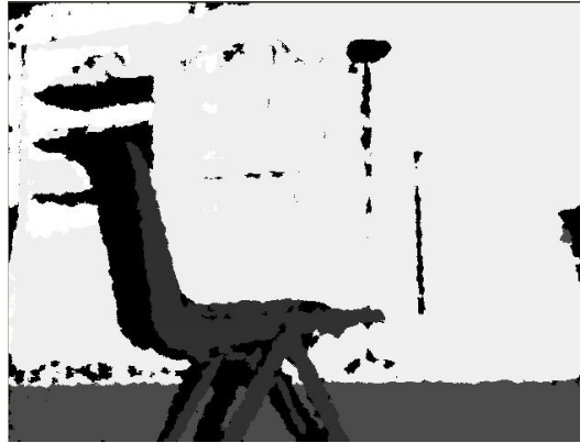
Figure 2. Depth image provided by the Kinect.
