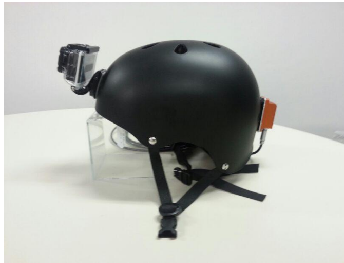
Figure 9. View of the helmet with the camera and AHRS unit placement detail.
