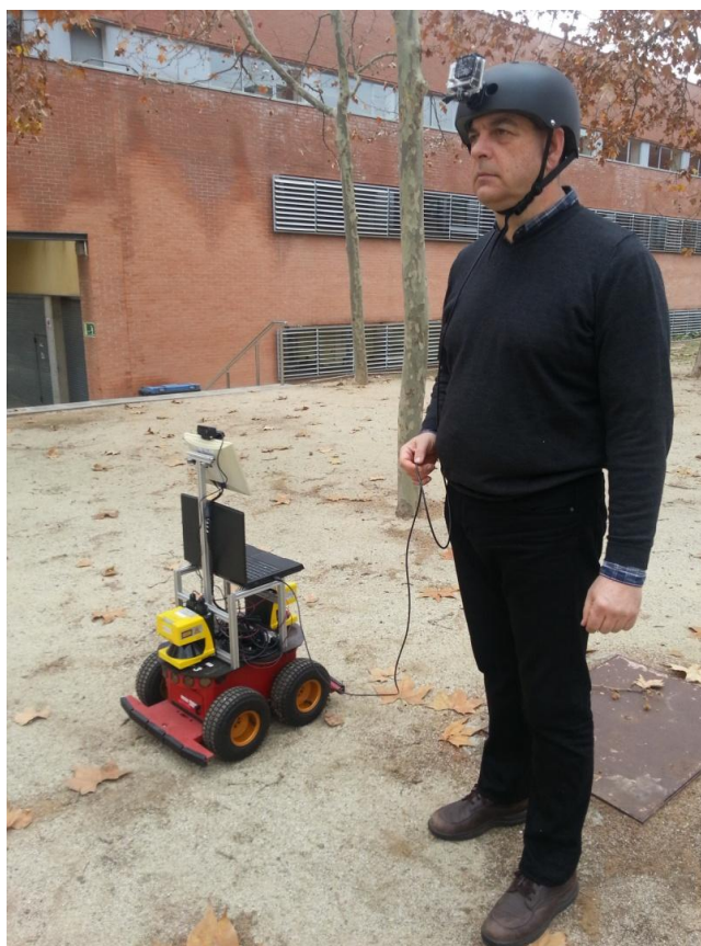
Figure 8. Robotic platform Pioneer AT3 with webcam and laser range finders. Helmet with camera and AHRS.
