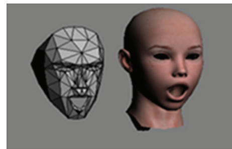
FIGURE 3: AU1—Jaw Lowerer Each AU is expressed as a numeric weight varying between -1 and +1 . This figure has been extracted from the Face Tracking SDK Kinect for Windows available at http://msdn.microsoft.com/en-us/library/jj130970.aspx .
