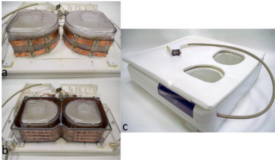
Fig. 1. Photograph of the 7-T bilateral coil: (a) dual solenoid with the cover and shield removed, (b) dual solenoid with shield, and (c) assembled coil
