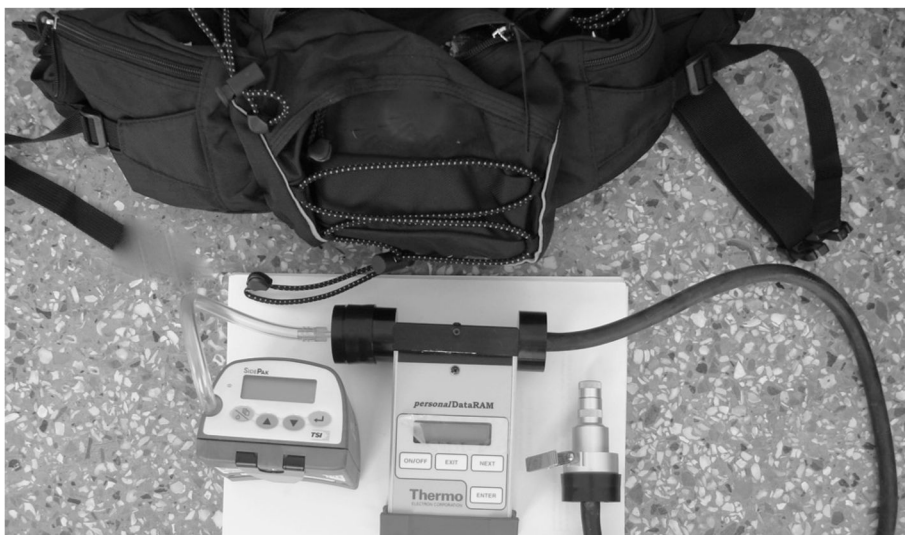
Photo 2. Personal air sampling system including Triplex cyclone, Personal Data Ram, battery operated TSI Sidepak SP530, and waist pack.
