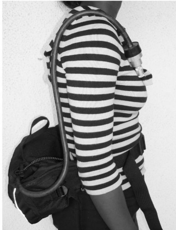
Photo 3. Personal air sampling system as worn by study participants. The Personal Data Ram and TSI Sidepak SP530 are fitted in waist pack while the Triplex cyclone remains near breathing zone.
