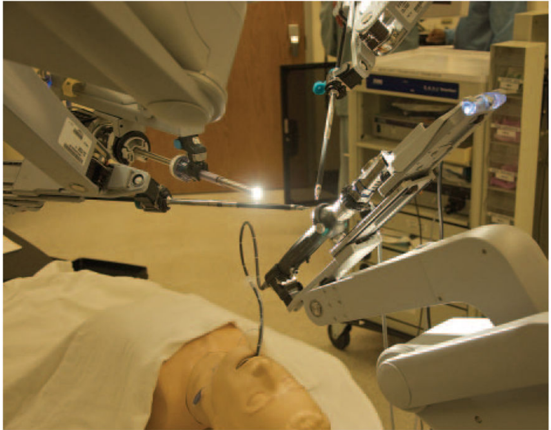
Figure 1. Schematic depicting the arrangement of the DaVinci Surgical System type S (DVS), bronchoscope, and airway mannequin.
