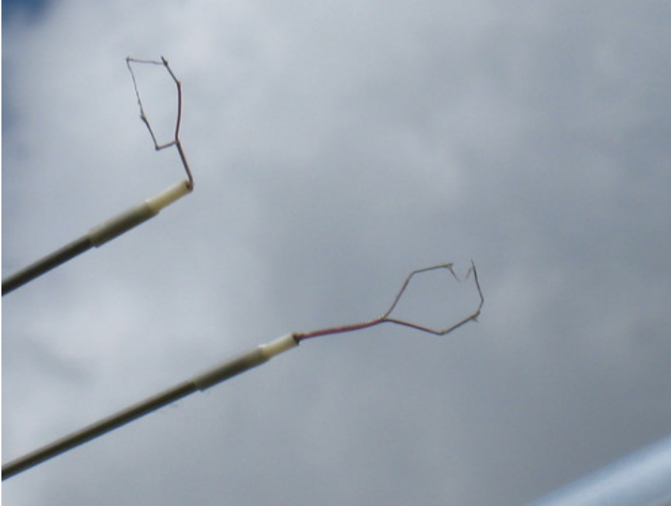
Figure 6. Fine wire chromel-constantan thermocouples (13 \mu\text{m} diameter) used for sensible heat measurements ( H ) in the surface renewal system.
