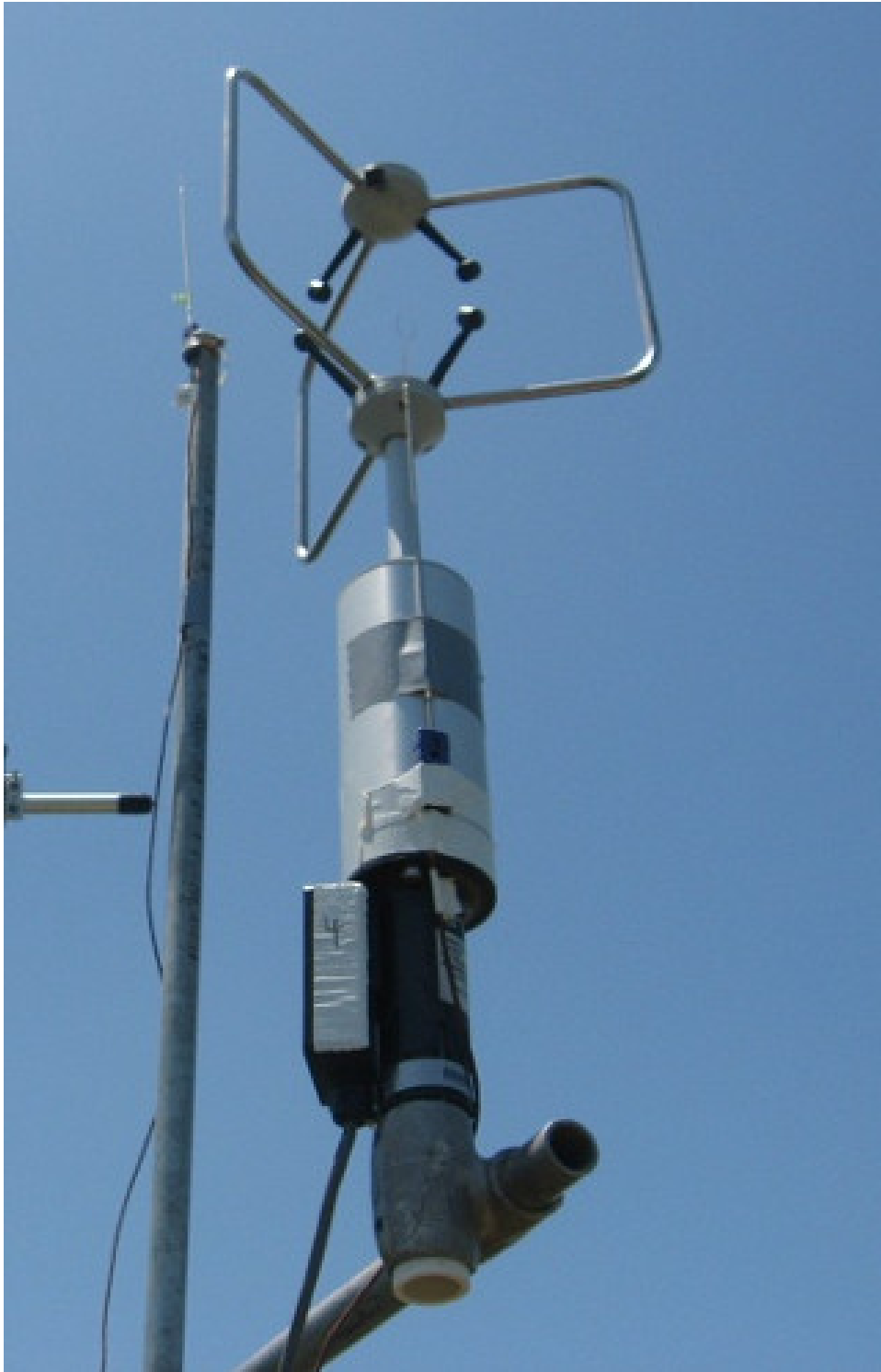
Figure 7. Sonic anemometer used for eddy covariance measurements to calibrate surface renewal. Instrument shown here is installed on a tower over a bare soil surface.
