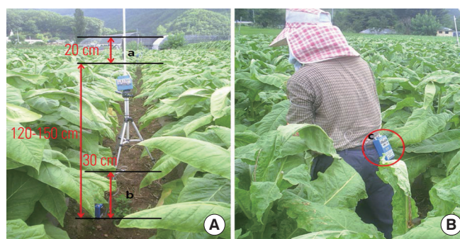
Figure 1. Samplers used to measure airborne nicotine concentrations in the tobacco field (A) and on the farmer (B). (a) Upper region, (b) lower region, (c) air sampler.
