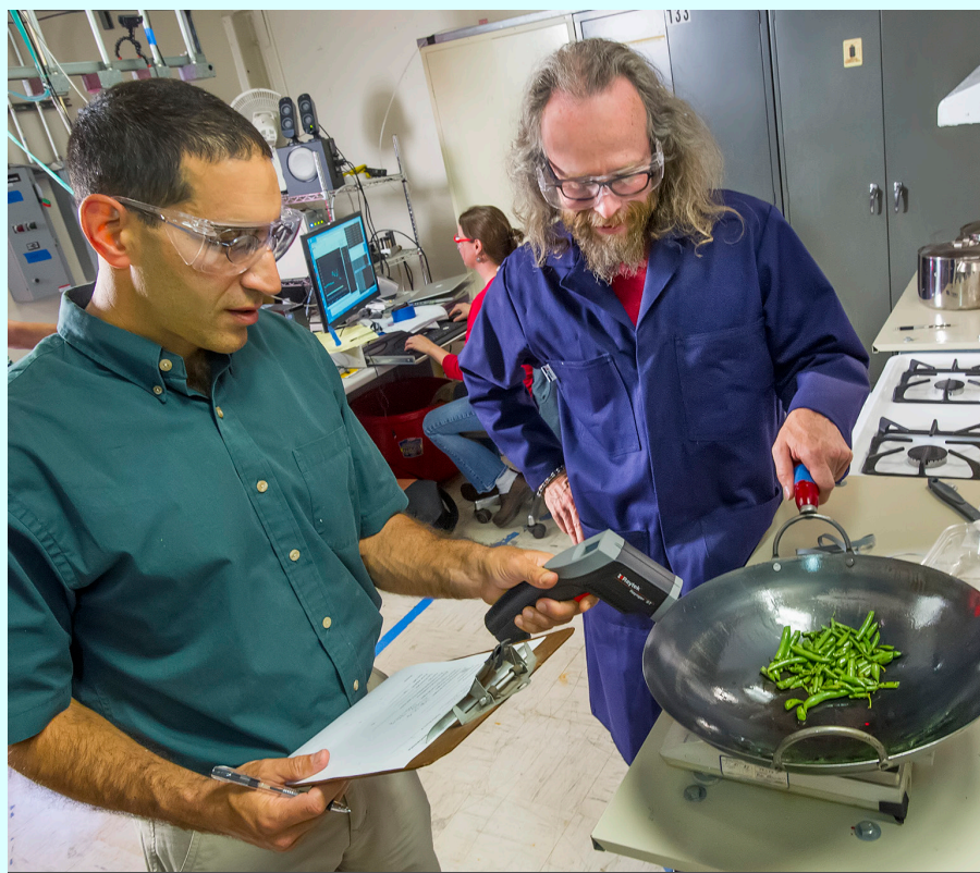
Tiny variations in cooking can dramatically affect emissions, so when researchers Brett Singer (left) and Woody Delp (right) study cooking-related pollutants, they take care to replicate temperature, fuel flow, cooking time, and other factors. Here, in their LBNL lab, Singer uses an infrared thermometer to ensure the temperature of the pan is the same during each standardized cooking event.
