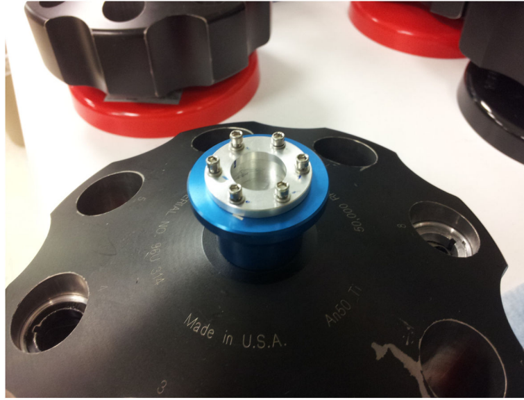
Figure 1. Photograph of the iButton holder in a modified rotor handle. A central cup is machined in a regular rotor handle such that the iButton is held in firm thermal contact with the rotor. It is secured in place with an aluminum ring fastened to the rotor handle with screws.
