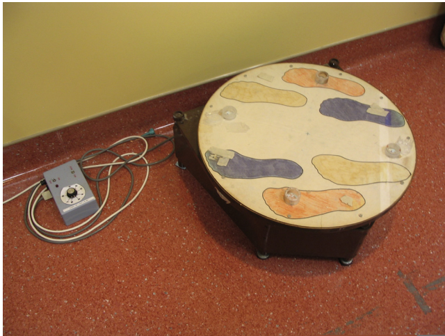
Fig. 20 – The custom built rotating platform with the three color-coded feet locations. A variable speed regulator is seen at the left of the platform.
