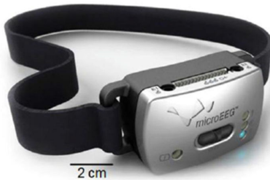
Figure 1. microEEG attached to a headband.
