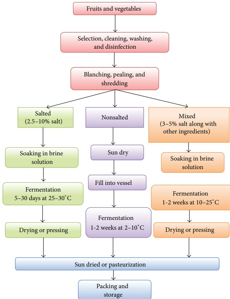
FIGURE 1: Overall fermentation process of fruits and vegetables.
