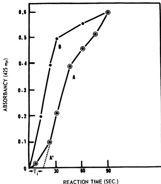
FIG. 1 (left). Time course of Enzymic peroxidation with two substrates. Curve A, eugenol; curve B, pyrogallol. Induction time, T<sub>i</sub>, is obtained from A', the extrapolated linear segment of A.
