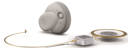
FIGURE 2: The Vibrant Soundbridge (VSB) implantable hearing device. The VSB system is comprised of two parts: the internal component is called the vibrating ossicular prosthesis (VORP) and the external component is an audio processor (AP). The VORP consists of a receiver coil, a magnet to hold the Amadé audio processor over the implant, a demodulator, the conductor link, and the floating mass transducer (FMT). The receiver coil sends the sound signal from the audio processor to the demodulator or electronics package. The demodulator demodulates the signal so that it can be converted into signals that will drive the FMT. The conductor link just sends these signals to the FMT. Adapted from marketing materials on the VSB, with permission of MED-EL, Innsbruck, Austria.
