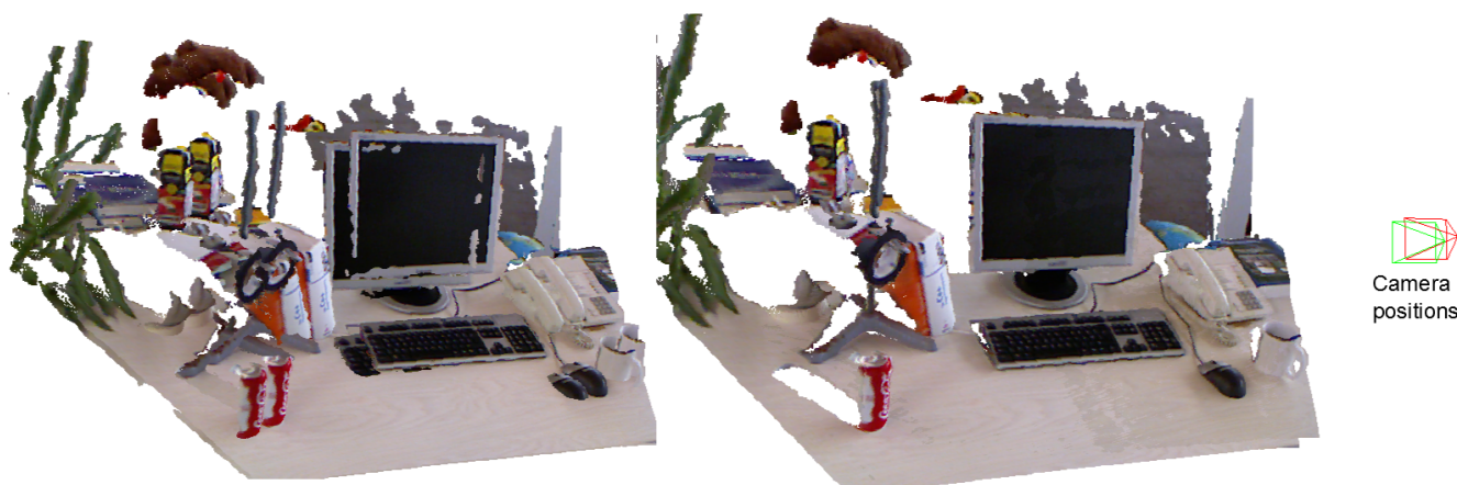
Figure 1. (Left) Two non-aligned point clouds. (Right) Both point clouds aligned and the estimated and reference positions of the camera.
