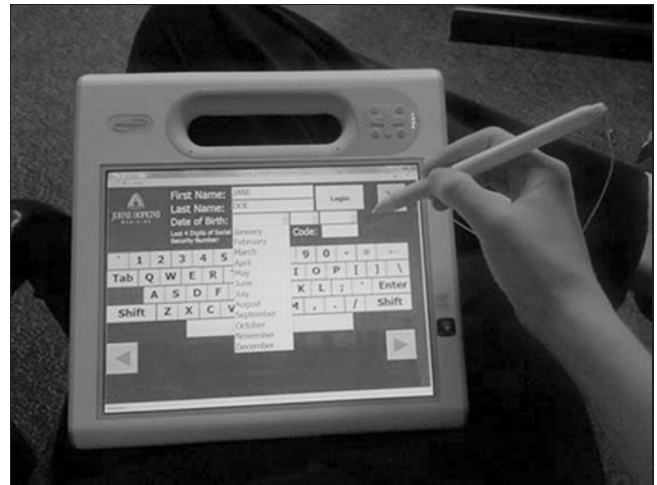
Fig. 1. Prototype kiosk: a computer tablet with pen-based touchscreen functionality used in the usability study with the login screen displayed.
