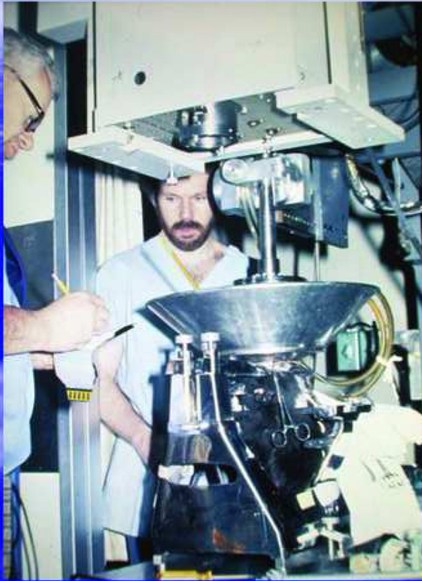
Figure 5. An early b-mode image guided HIFU system designed in the 1970's by the Fry brothers to treat brain cancer patients.
