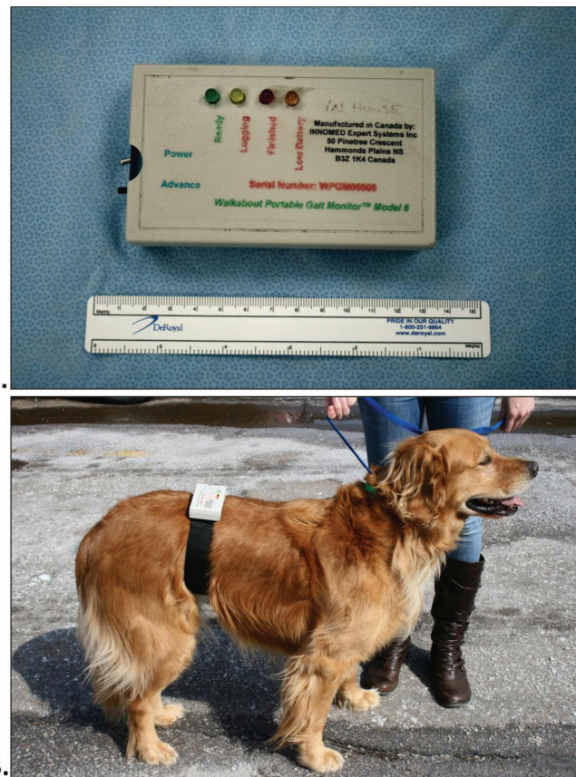
Figure 1. Walkabout Portable Gait Monitor (WPGM) alone (A) and positioned over the mid-lumbar spine of a dog (B). This is a triaxial accelerometer system that measures acceleration in the 3 cardinal planes and is used to obtain kinetic and kinematic gait data.
