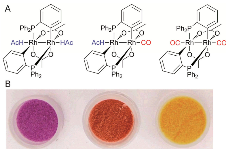
Fig. 4. Colourimetric detection of CO via binuclear rhodium complexes. (A) Basic structure of the complexes (HAc = CH 3 CO 2 H). (B) The photograph shows ([Rh 2 {( m -CH 3 C 6 H 3 )P( m -CH 3 C 6 H 4 ) 2 } 2 (O 2 CCH 3 ) 2 ](CH 3 CO 2 H) 2 ) adsorbed on silica gel in the absence (left) and presence of 8 ppm (middle) and 2000 ppm (right) of CO. Adapted and reprinted with permission from ref. 110 Copyright 2011 American Chemical Society.
