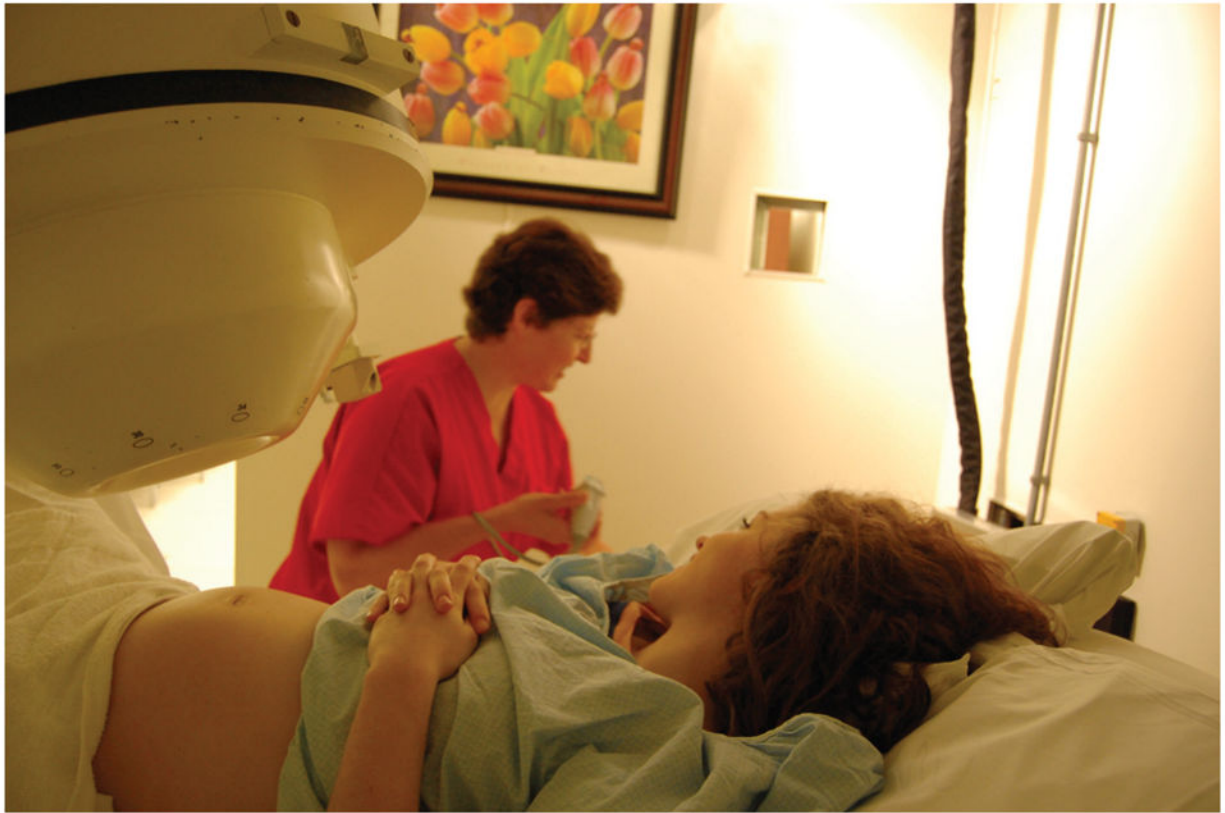
Fig. 2. Dr. Strasburger performing ultrasound within the magnetically shielded room at UW-Madison Biomagnetism Laboratory, The superconducting quantum interference device above the patient is not yet in position against the maternal abdomen.
