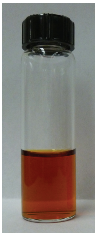
Figure S4 Picture of a dispersion of N-(trimethoxysilylpropyl)ethylenediaminetriacetate-iron oxide nanoparticles in water.
