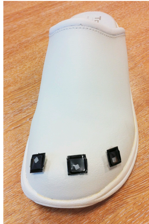
Figure 1. A theatre clog showing the type and location of the thermoluminescent dosimeters. For clarity these are shown on the exterior of the clog but were inside for the in situ monitoring.
