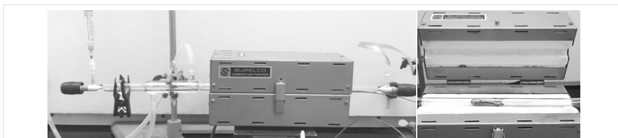
Figure 8: Tubular reactor used in the catalytic reduction reaction.
