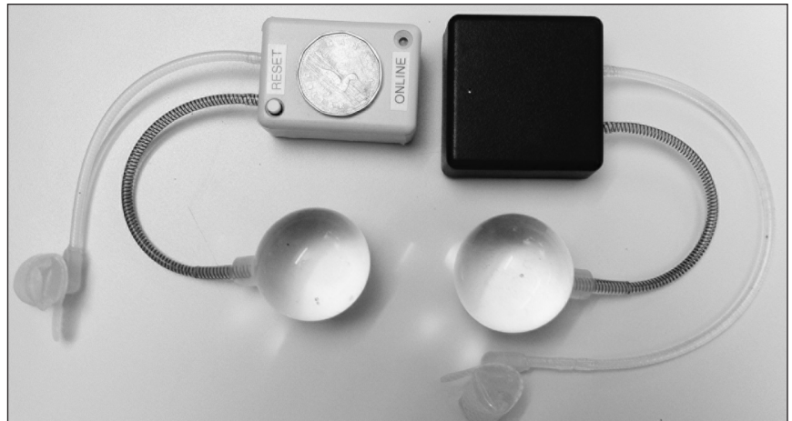
Fig. 10. The novel, remotely-controlled artificial urinary sphincter.
