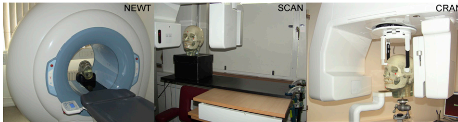
Figure 1 The unit's chair was not used unless its control was isolated from the cone beam CT unit [as was the case for NewTom™ 5G (NEWT; QR Srl, Verona, Italy)]. For Scanora® 3D (SCAN; Soredex Oy, Tuusula, Finland) i-CAT (Imaging Sciences International, Hatfield, PA) and 3D Accuitomo FPD80 (Morita, Kyoto, Japan) a table with adjustable height together with a wooden plate (used as an extension) served as support for the skull, whereas for Cranex® 3D (CRAN; Soredex Oy) and Promax® Dimax 3 (Planmeca Oy, Helsinki, Finland), a tripod was used to support the skull.
