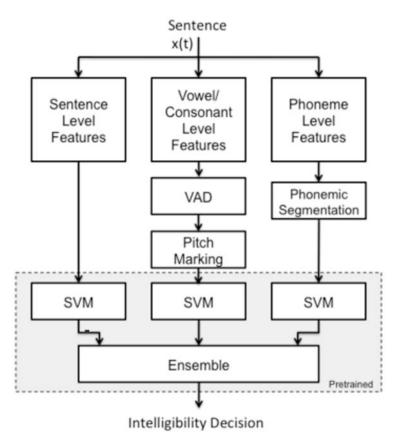
**Figure 1.**A high-level diagram of the proposed classification framework. Features are extracted at three different scales, and a final intelligibility decision is made by combining individual decisions from each scale.
