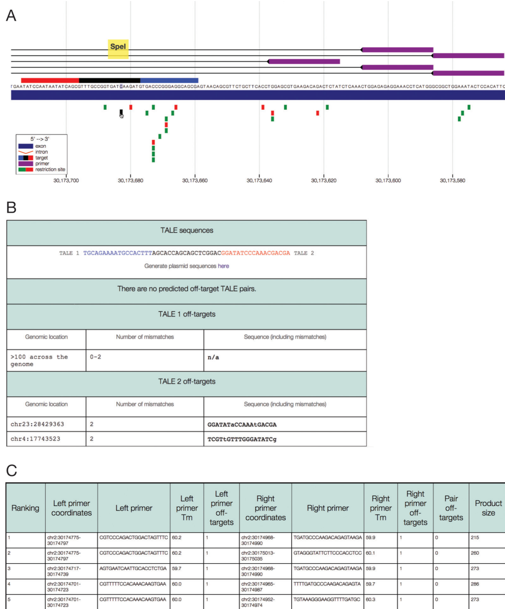
Figure 2. CHOPCHOP provides detailed information about each CRISPR/Cas9 and TALEN target site. (A) The detailed information page provides a zoomed in view of the target locus with visible DNA sequence, primer options (above the gene, purple) and restriction sites (below the gene; green if unique in the region, red if not). In TALEN mode the target site is color-coded; TALEN 1 is blue, the spacer is black and TALEN 2 is red. (B) Information is provided about predicted off-targets: the genomic location, number of mismatches and location of mismatches within the sequence. (C) Information is provided about the primer designs, including the primer sequence, T_m and product size.
