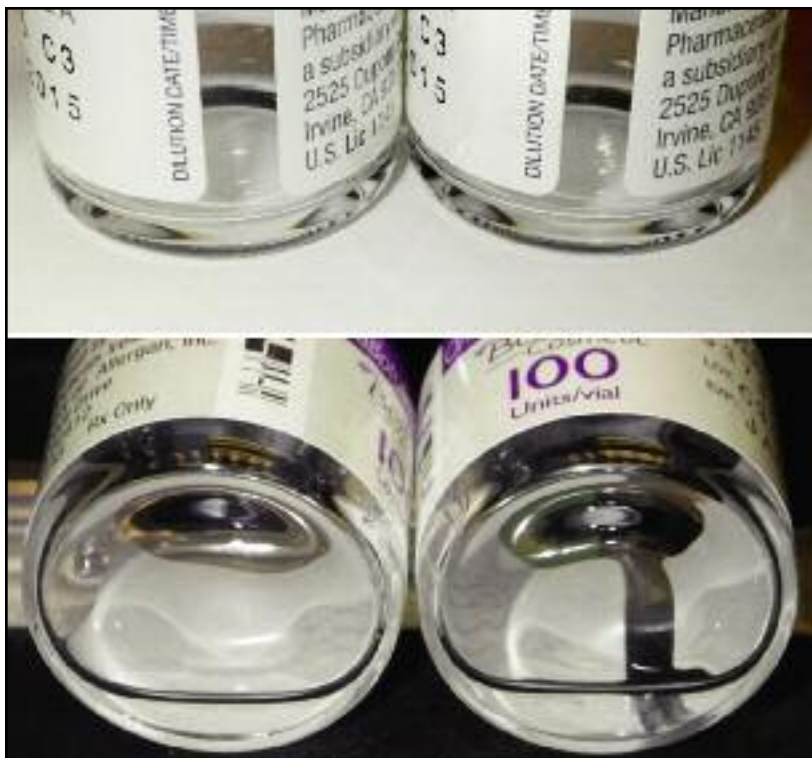
Figure 2. A flat and level vial may appear as if it has no residual liquid in it (top), while a tilted vial will better show any residual (bottom).
